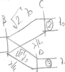
$$S_{11} = \left| \frac{b_1}{a_1} \right|_{a_2 = a_3 = 0} = \frac{V_0^+}{V_A^-}$$
