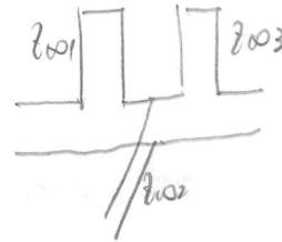
$$\text{dove } Z_{001} = R_o g_1 ; Z_{002} = \frac{R_o}{g_2} ; Z_{003} = R_o g_3 ;$$
