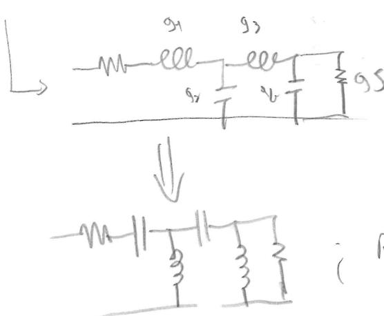
$$j\omega b \rightarrow -j \frac{w_b}{\omega} l = \frac{l}{j\omega c} \quad l = \omega_c l$$
