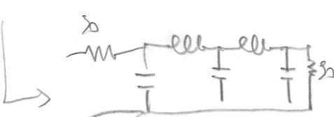
$$a = \frac{\omega_0}{R_0}; l_2 = g_2 R_0; c_3 = \frac{g_3}{R_0}; l_4 = g_4 R_0; c_5 = \frac{g_5}{R_0};$$
