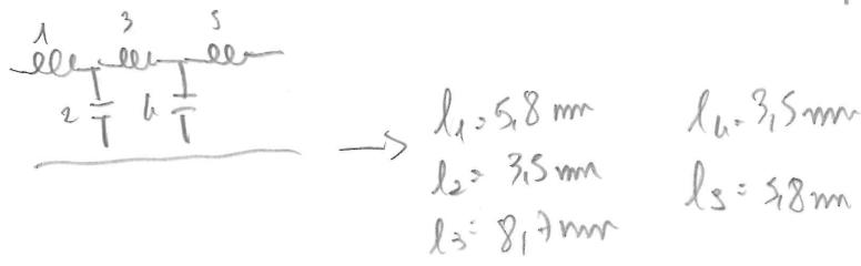
$$8.20) N=4; \text{ bandstop; open-circ quarter-wave; } f_0 = 3 \text{ GHz}, D = 0.15, R_o = 60 \Omega$$
