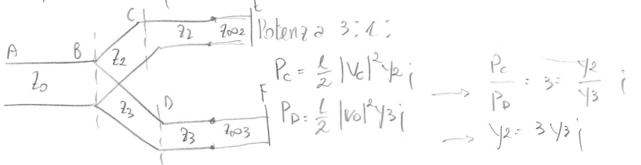
$$\rightarrow y_0 = y_2 + y_3 = 4y_3 \rightarrow y_3 = 8.3 \text{ mS} ; z_3 = 120 \Omega ; z_2 = 40 \Omega$$
