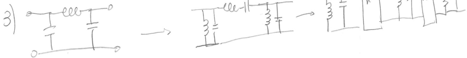
$$j\omega e \rightarrow j \frac{l}{\delta} \left[ \frac{\omega}{\omega_0} - \frac{\omega_0}{\omega} \right] e = \underbrace{\frac{l}{\delta} j \frac{\omega}{\omega_0} e}_{j\omega C} - \underbrace{\frac{l}{\delta} j \frac{\omega_0}{\omega} e}_{j\omega L} \rightarrow \frac{l}{L} = \frac{l}{\delta} \frac{\omega_0}{\omega} \frac{gm}{B} \quad L = \frac{\Delta R_o}{\omega_0 gm}$$
