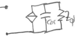
$$\Rightarrow jX_{C_{DS}} = \frac{1}{j\omega C_{DS}} = \frac{1}{j56 \times 0,3} = -j106,1 \Omega; jB_{C_{DS}} = 9,1425 mS.$$
