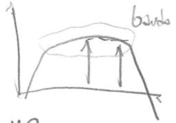
CIM<sub>3</sub>: carrier to IM<sub>3</sub>: differenza in dBc tra la portante e i IMP<sub>3</sub>.
